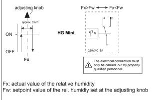
If the rel. humidity Fx (actual value) falls below the setpoint value Fw, contact 1/4 opens and contact 1/2 closes.
